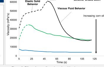
Figure 4: Effect of corn oil on yield stress of fresh state concrete
