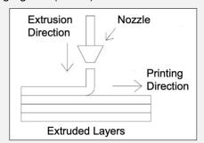
Figure 2: General scheme of 3D printing concrete[1]
