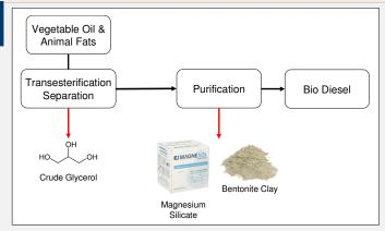
Figure 3: Biodiesel production scheme and desired waste materials<sup>[2]</sup>
