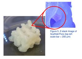
Figure 4. 3D Printed Bone Scaffold
