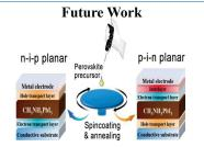
Figure 8. Visual of MAPbI3 device stack structures4.
