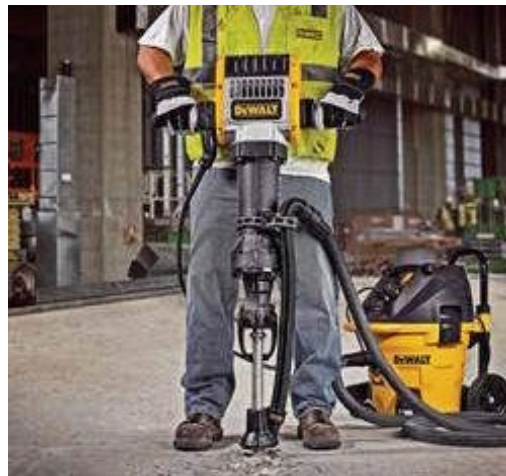
Jackhammer equipped with VDCS. Shroud around hammer connects to the vacuum on the right.
