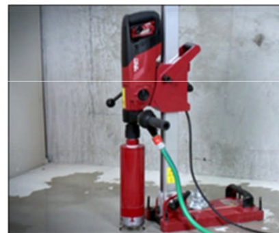
Example of a core saw with integrated water delivery system.
