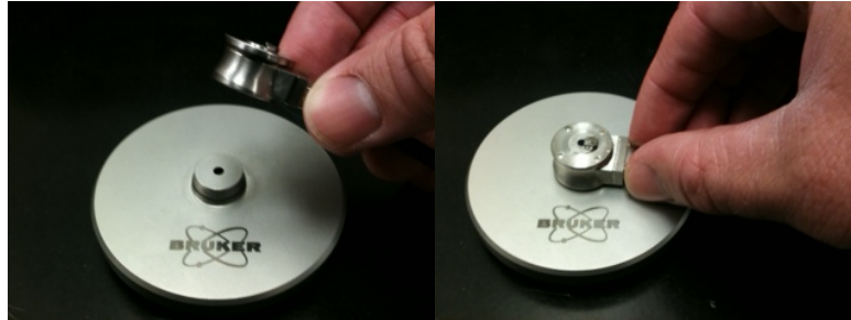
Figure 1. The FastScan probe holder (also known as the FastScan Z scanner) and probe holder mounting block for the Dimension FastScan AFM.
