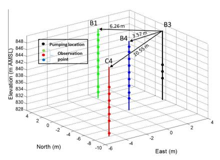
Fig. 2. The setup of pumping tests at the BHRS. Pumping is conducted in Well B3 and observation points are in Wells B1, B4 and C4.
