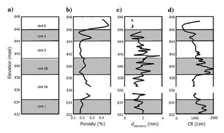
Figure 3. Profiles at borehole C4: (a) unit boundaries, (b) porosity, (c)  $d_{60}$  for the matrix only ( $d_{60[\text{matrix}]}$ ), and (d) CR. Sources: Barrash and Clemo (2002), Reboulet and Barrash (2003), Mwenifumbo et al. (2009), and Barrash and Cardiff (2013).
