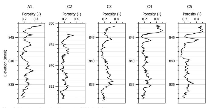
Figure 2. Example porosity profiles from central well field borehole logs.
