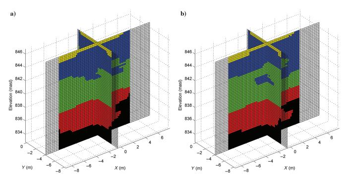
Figure 11. Results of five-cluster analysis showing (a) clusters based on real conductivity and (b) clusters based on real and imaginary conductivities.
