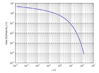
**Fig. 13.** The attenuation of the signal with  $\gamma$ .  $h_0 = \frac{Q}{2\pi T}$ . Note that at  $\gamma \approx 100, h \approx \frac{Q}{2\pi T} * 10^{-3}$ . With typical values of Q = 0.1 (L/s) and  $T = 10^{-4}$  (m<sup>2</sup>/s), the signal for  $\gamma = 100$  would be  $h \approx 2 * 10^{-4}$  (m).
