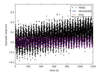
**Fig. 5.** Hydraulic head at the entire sampling duration, in the case of white noise with a linear drift.  $n \sim \mathcal{N}(0, \sigma^2)$  and a linear drift  $\alpha = 0.01$  (cm/s).  $\sigma = 5$  (cm) (left). The  $L^2$  norm of the relative error is 1.7% and the root mean square error of the estimates is 0.06 (cm) and (right) plot of the root mean square error with time. The data is synthetic, with the true signal being that shown in (13).
