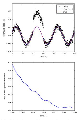
**Fig. 3.** Hydraulic head at three periods, in the case of white noise with an abrupt shift of half a period (The jump is exaggerated for illustration purposes).  $\epsilon \sim \mathcal{N}(0, \sigma^2), \sigma = 1$  (cm) (top). The  $L^2$  norm of the relative error is 2.8% and the root mean square error of the estimates is 0.1 (cm) and (bottom) plot of the root mean square error with time. The data is synthetic, with the true signal being that shown in (13).
