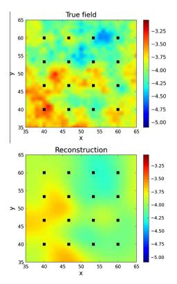
**Fig. 9.** The true log transmissivity field (top) and the reconstructed log transmissivity field (bottom). The relative  $L^2$  error within the area of measurements is 0.18 – for the joint inversion. The plots are zoomed in so the area of measurements is more clearly visible.
