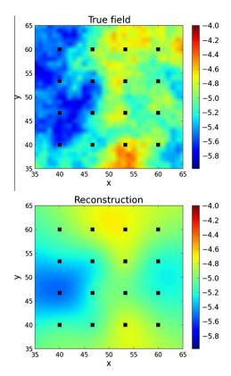
**Fig. 10.** The true log storativity field (top) and the reconstructed log storativity field (bottom). The relative  $L^2$  error within the area of measurements is 0.59 – for the joint inversion. The plots are zoomed in so the area of measurements is more clearly visible.
