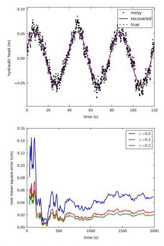
**Fig. 6.** Hydraulic head at three periods, in the case of AR (1) noise. AR (1):  $\epsilon_i = c\epsilon_{i-1} + n_i$ , where  $n_i \sim \mathcal{N}(0, \sigma^2(1 - c^2)), \sigma = 1$  (cm), c = 0.8 (top). The  $L^2$  norms of the relative error is 1.1% and the root mean square error is 0.04 (cm) and (bottom) plot of the root mean square error with time for various correlation coefficients. The data is synthetic, with the true signal being that shown in (13).
