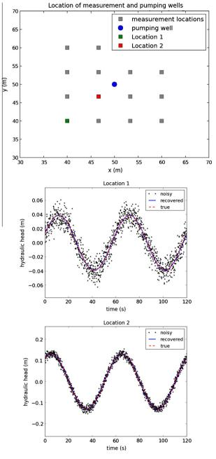
**Fig. 7.** (top) The location of the pumping source and the measurement wells and (middle, bottom) the synthetic generated signal used for the inverse problem, noisy and denoised, at two locations.
