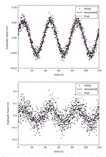
**Fig. 1.** Hydraulic head at three periods, in the case of white noise.  $\epsilon \sim \mathcal{N}(0, \sigma^2)$  with  $\sigma = 1$  (cm) (top) and  $\sigma = 5$  (cm) (bottom). The  $L^2$  norm of the relative errors are respectively 0.36% and 1.7%. The root mean square errors in the estimates are respectively 0.01 (cm) and 0.06 (cm). The data is synthetic, with the true signal being that shown in (13).
