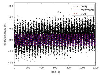
**Fig. 4.** Hydraulic head at the entire sampling duration, in the case of white noise with a linear drift.  $n \sim \mathcal{N}(0, \sigma^2)$  and a linear drift  $\alpha = 0.005$  (cm/s).  $\sigma = 5$  (cm) (top). The  $L^2$  norm of the relative error is 2.9% and the root mean square error of the estimates is 0.1 (cm) and (bottom) plot of the root mean square error with time. The data is synthetic, with the true signal being that shown in (13).
