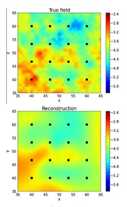
**Fig. 8.** The true log transmissivity field (top) and the reconstructed log transmissivity field (bottom) the relative  $L^2$  error within the area of measurements is 0.13 – for the inversion for transmissivity only. The plots are zoomed in so the area of measurements is more clearly visible.
