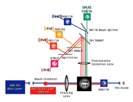
Figure 4-1 Optical bench diagram of the FACSCalibur benchtop flow cytometer
