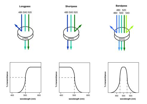
Figure 4-4 Light transmittance through longpass, shortpass, and bandpass filters
