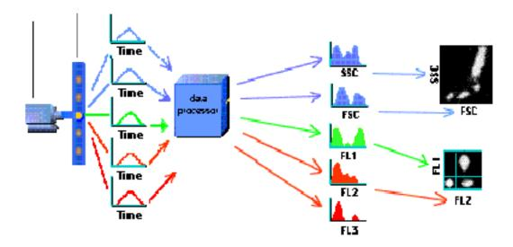
**Figure 1-1** Scattered and emitted light signals are converted to electronic pulses that can be processed by the computer
