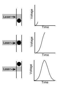
Figure 4-5 Creation of a voltage pulse
